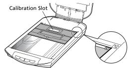
Align the Film Guide's 🗔 mark with the scanner's 🏻 mark.
